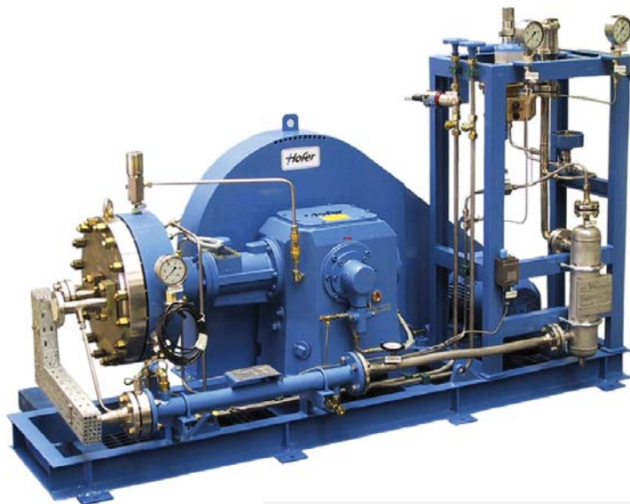
Single-stage diaphragm compressor Model: MKZ 400-5 Capacity: 74 scfm (~125 Nm 3 /h) Suction pressure: 203 psi (14 bar) Discharge pressure: 450 psi (31 bar)
