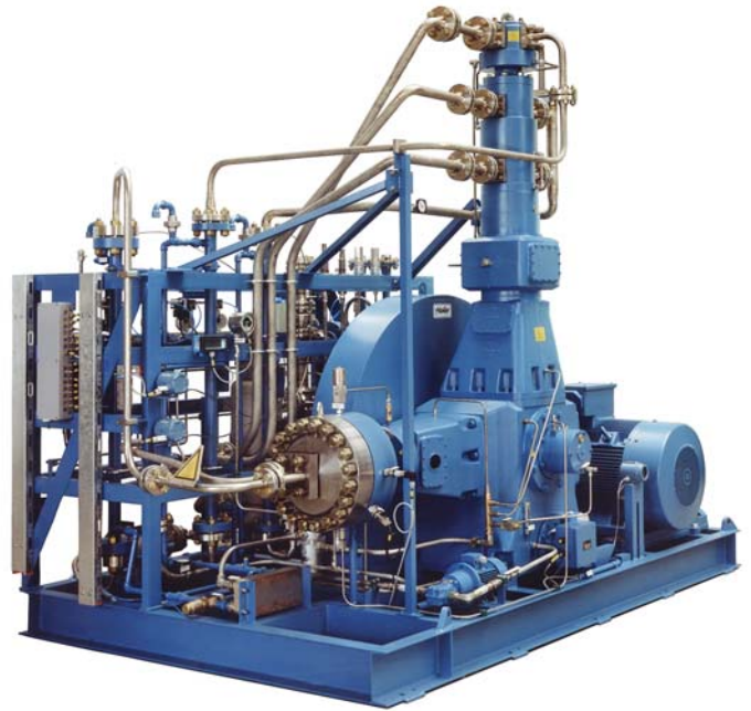
2-stage dry running piston compressor with final diaphragm stage Model: 120TK500 / MKZ 350-40 Capacity: 295 scfm (~500 Nm 3 /h) Suction pressure: 232 psi (16 bar) Discharge pressure: 4.350 psi (300 bar)
